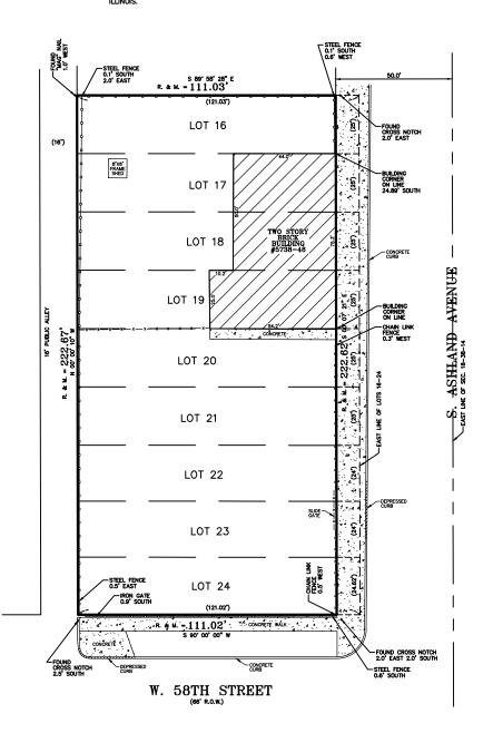
NOTE: R. & M. DENOTES RECORD AND MEASURED DISTANCES RESPECTIVELY BEARINGS SHOWN HEREON ARE MEASURED
